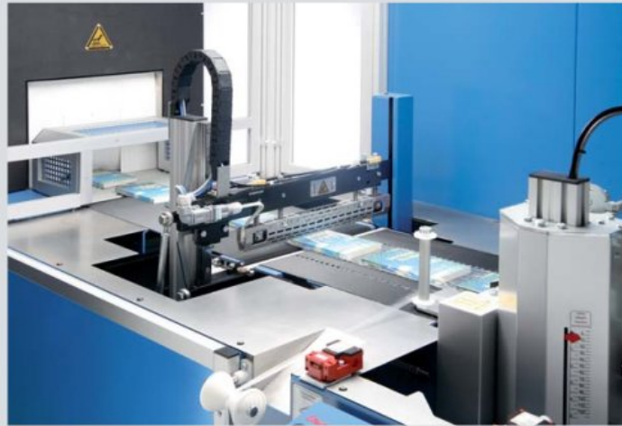
Continuous motion sealing jaw driven by servo guarantees no empty bags.
